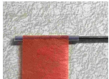
When ready to roll the tube, turn the mandrel/tissue over so the tissue is underneath the Teflon. Run glue along the Teflon tube and down the sides at least 1/3 of the way down the strip.
